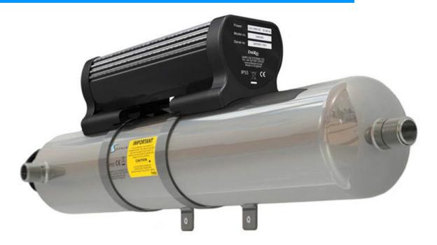
The Saphir system is a compact, economical UV system that is designed with the consumer in mind. The Saphir system utilises commonplace single ended low pressure UV lamp technology, thus making the system not only economical for energy running costs, but also for replacement UV lamps. The single ended UV lamp also makes servicing the equipment very simple. All systems comply with international UV dose standards and are designed to meet these standards even at end of lamp life.
